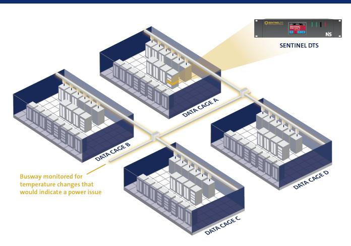
The SENTINEL TS attaches optical fiber directly to powerbusways to enable continuous, real-time temperature monitoring along their entire length. Using Raman scattering to analyze backscattered light in the fiber, it accurately detects overheating patterns
